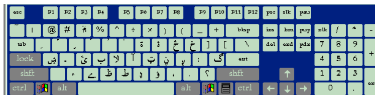
Fig 6.2 shift state keyboard layout
