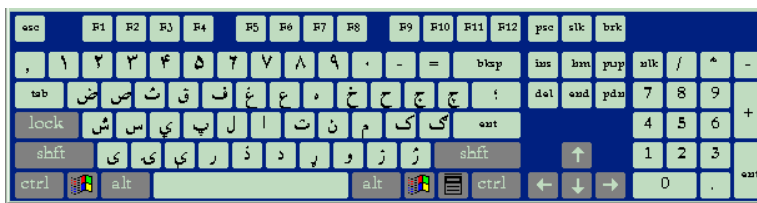
Fig 6.1 normal state keyboard layout
